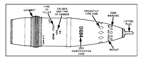
PROJECTILE, 8-INCH: ICM, M404. These projectiles are improved conventional munitions (ICM) used primarily against personnel. The projectile has the same external configuration and ballistic characteristics as the M106 and is provided with a fusible lifting plug (yellow). The cargo consist of 104 M43A1 antipersonnel grenades which are expelled from the projectile in flight when a preset fuze ignites an expulsion charge. The projectile spin centrifugally disperses the grenades from the projectile
