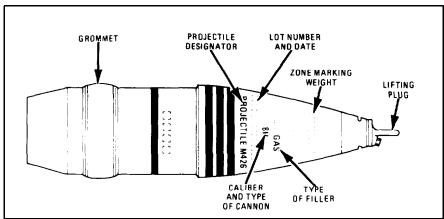
PROJECTILES, 8-INCH: GAS, NONPERSISTENT, GB, M426 AND GAS, PERSISTENT, VX, M426. These projectiles are used as casualty producing agents. The projectile is similar in configuration to HE Projectile M106. It is composed of a steel forging fitted with steel burster case, a nose adapter, and a gilding metal rotating band. The burster case contains a burster loaded with
